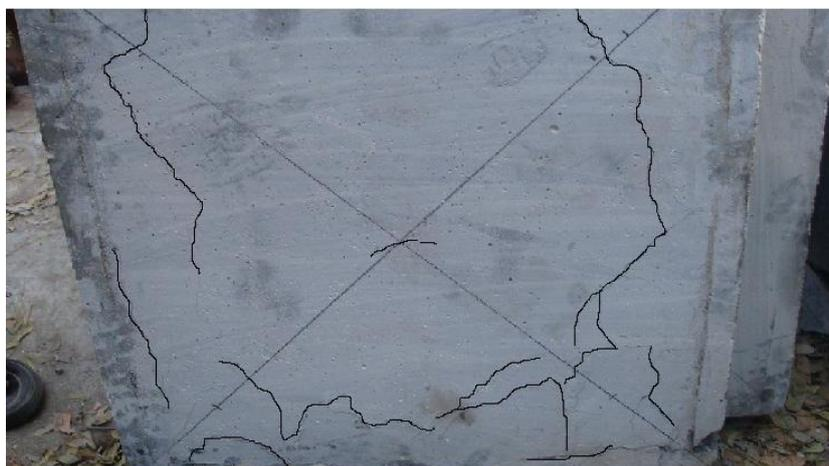
**Plate 1. Crack Pattern of slabs**
