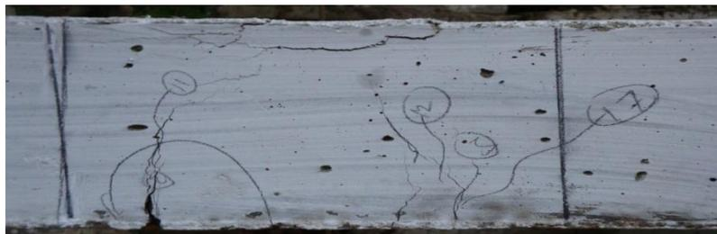
**Plate 1. Crack Pattern of Beam**
